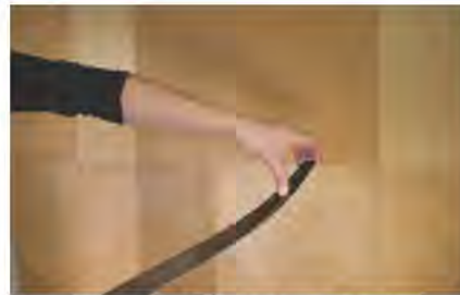
Figure 10: Bending the saw with the hand
