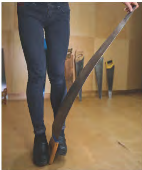
Figure 7: Standing and holding the saw in between the feet.
