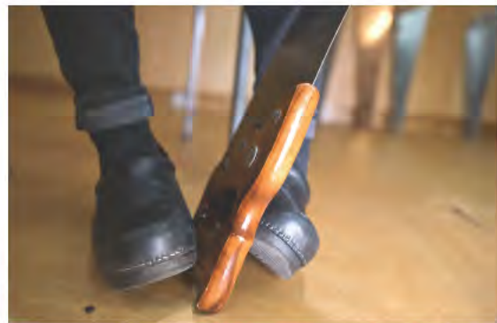
Figure 6: Sitting and holding the saw between the feet.
